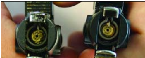
Clogged Flame Holes
