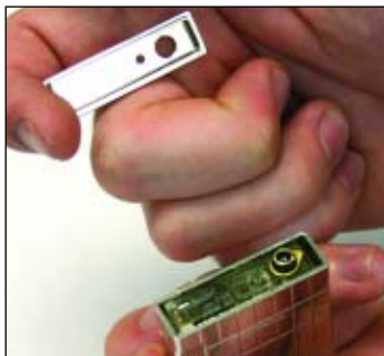
2. Pull out the bottom cover from the lighter to get to the O-Ring and Stopper.
