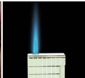
6. Check the flame height before you put the Stopper, O-Ring and bottom cover back together.
